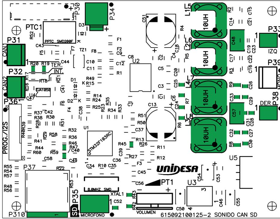
NOTA : R6, R7, R8, R9, R19, R20, R42, R43, R45, R46, R47, C24, C25, C26, C27, C28, C29, C30, C31, C32, C33, C48, C52, C57, L3, L4, L5, L6, L7, L8, P31, P32, P34, P35, P33, P38 y P310 no se montan.
