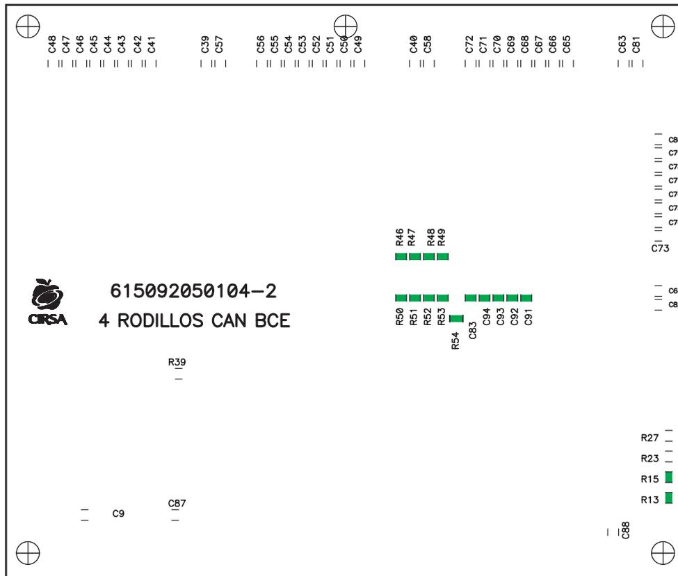
Nota: U9, R3, R4, R5, R6, R7, R13, R14, R15, R16, R17, R40, R46, R47, R48, R49, R50, R51, R52, R53, R54, C2, C4, C27, C28, C29, C30, C83, C91, C92, C93, C94, J1, J2, J3, J4, J5, LED1, LED2, LED6, P412, PTC1, PTC2, P41, P43 y P48 no se montan. Cód: 2050104-2
