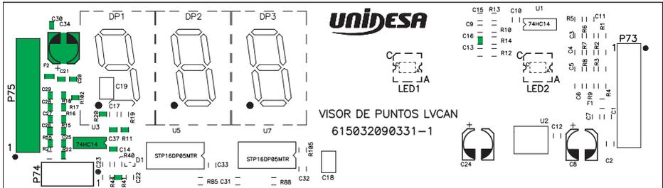
NOTA: C14, C16, C20, C21, C25, C26, C27, C28, C29, C30, C34, C37, F2, P75, R11, R15, R16, R17, R18, R20, R22, R44, R55, R102 y U3 no se montan.
