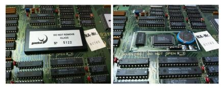
Under the cover is the RAM on the left, the DS5002FP in the middle, and the 3V lithium cell on the right. In front is a UART connector, which can be used to push new firmware to the system. That will generate a new key, so it is not useful in this attack.
